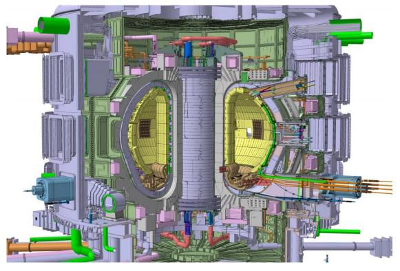
The ITER machine is based on the tokamak concept of magnetic plasma confinement, in wich the fusion fuel is contained in a doughnutshaped vessel. With a height of 29 m and a diametre of 28 m, ITER will be the worlds largest tokamak (ITER Organization -COM\_IMAGE\_DOWLOAD)
